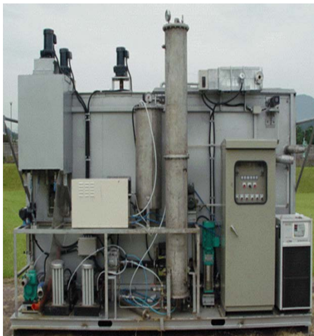
This photo shows Michigan Technology's Dissolved Ozone Flotation (DOF) Small Plant which can supply drinking water to approximately 1,000 persons. (Photo provided by company)
