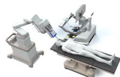
Flexible surgical robot (for endoscopic cancer surgery) A prototype is currently under development
