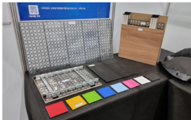
Photo 1. Wave META used for reducing NVH of EVs (left) and Wave META used for reducing noise between floors (right)
